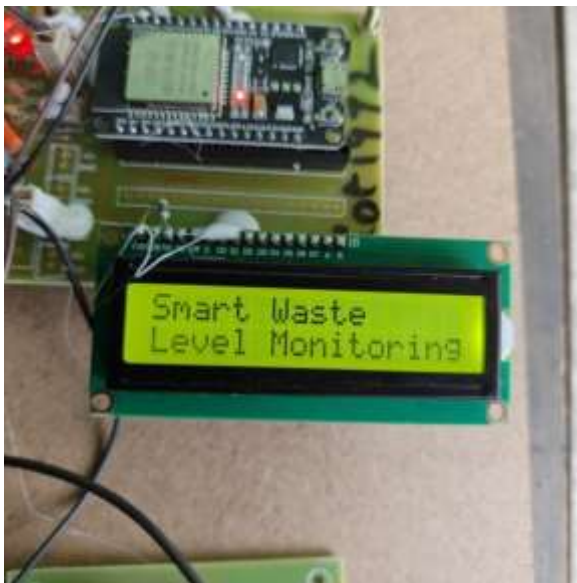
Fig. 3: LCD Display Showing Waste Level and System Status
