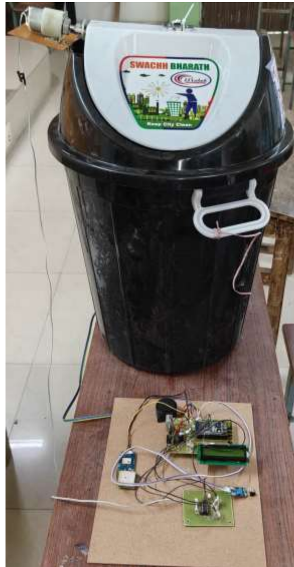
Fig. 4: Complete Smart Waste Bin Prototype with Integrated IoT System
