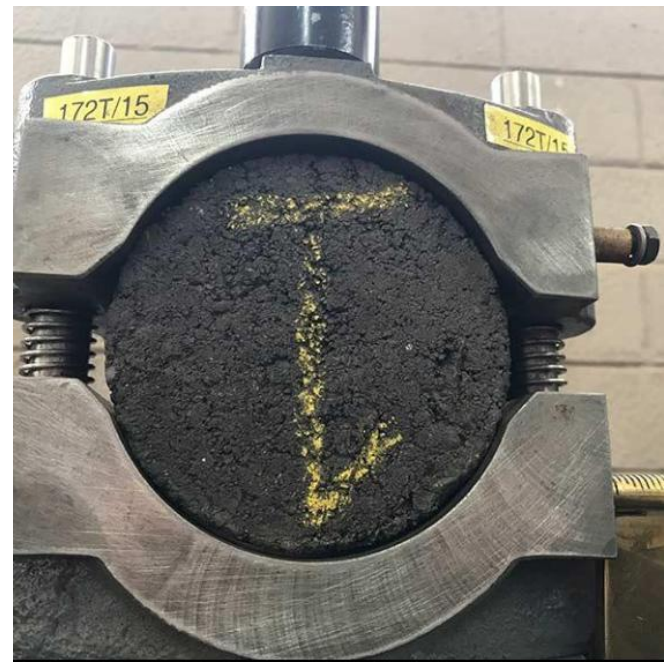
Figure 4. Marshall Stability Test of Modified Bituminous Mix
