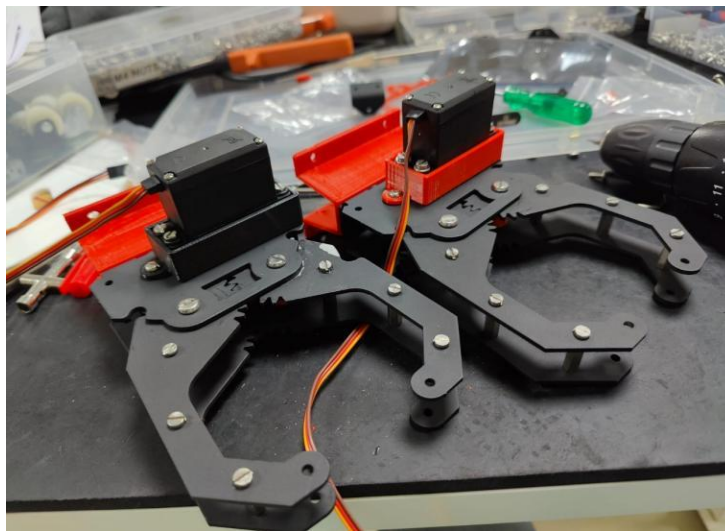
Figure. 4: Dual Servo Motor Gripper Mechanism for Robotic Manipulation
