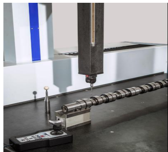
Fig. 4 Coordinate Measuring Machine (CMM) Inspection
