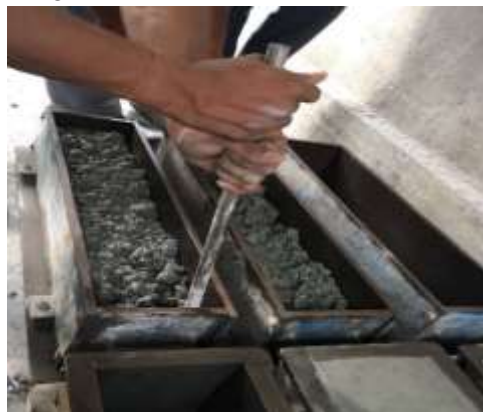
Compacting the concrete in the cube mould
