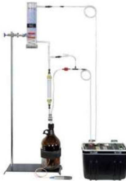
Fig 4: Typical set-up of RAD7 electronic radon detector
