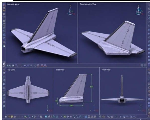
Fig. 2. Solid model of a fin blade with several perspectives.
