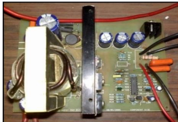
Fig 9: Boost converter hardware design
